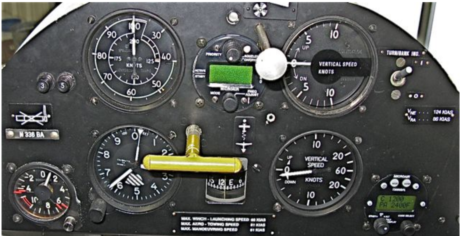
Mission complete! Below, note my new transponder (lower right) and new 720-channel radio (upper center).
